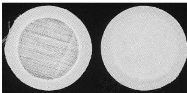
Figure 2 Coating of textiles with sol gel can improve the abrasion resistance as can be seen by comparing the result of Martindale Testing (EN ISO12947 - part 2) after 100.000 cycles on an untreated (left) and treated (right) woven PES substrate.
