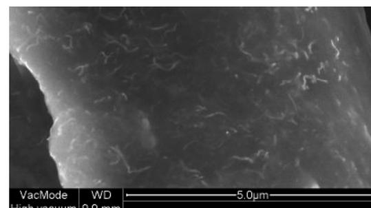
Figure 1 Coating of textiles with a CNT containing formulation: if aggregation of CNT occurs, this becomes visible as micrometer-sized dark spots (up); if well-dispersed these spots are prevented and via SEM analysis the individual CNTs can be seen (down).
