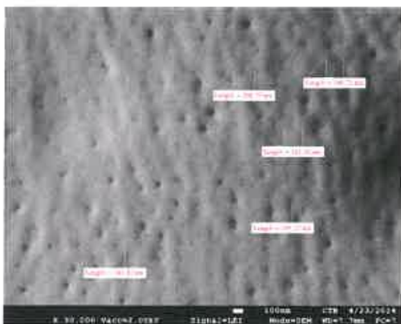
FIGURE 9: SEM image from the surface of an acrylate-based coating dried at 30°C with indication of the acrylate particle size.
