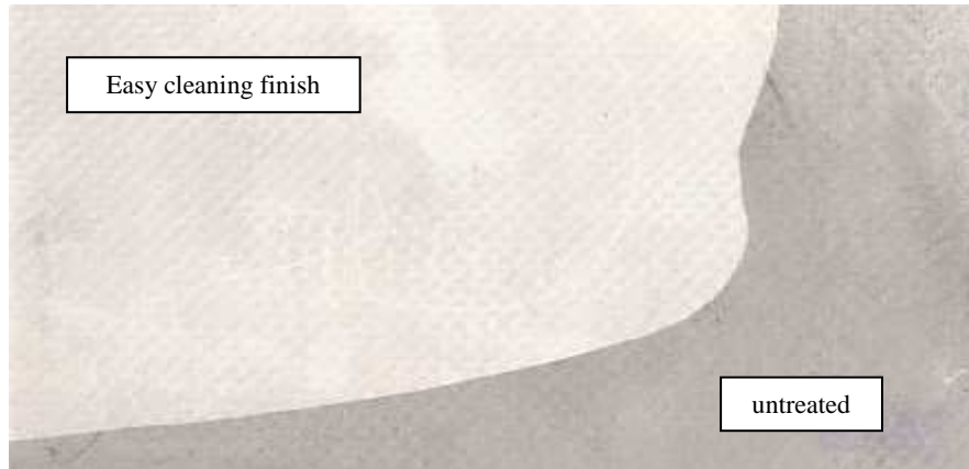
Figure 1: Soiled and cleaned membrane which is partially treated with the new topcoatings.
