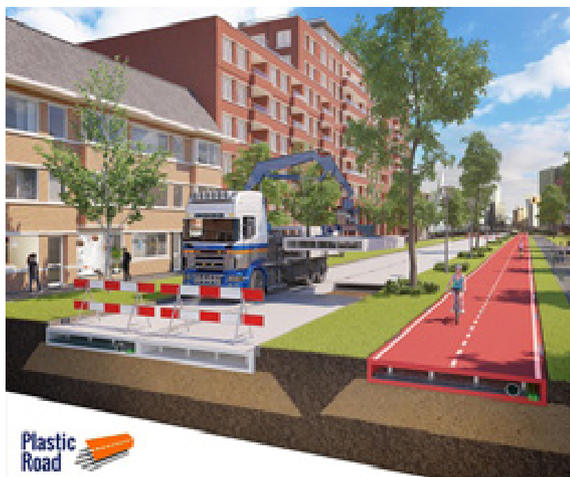
PlasticRoad structure enables various infrastructure elements to be incorporated, and is inherently recyclable.
