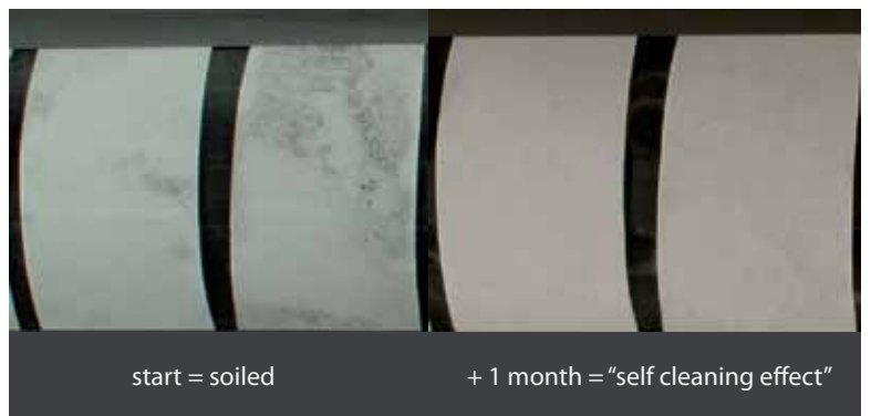
test results on self-cleaning coating (Contex-T)
