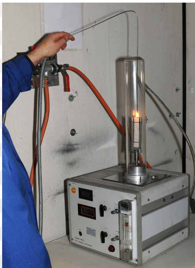
Limiting Oxygen Index (LOI) test
