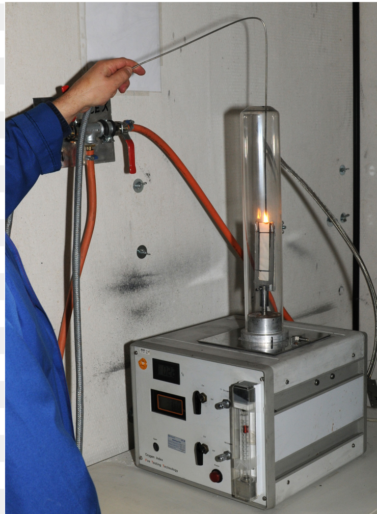
Essai "Limiting Oxygen Index" (LOI)
