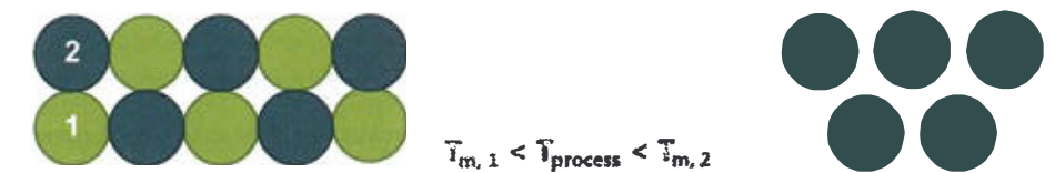
Fig. 2 Production of self-reinforced composite (1: low Tm PLA, 2: high Tm PLA)
