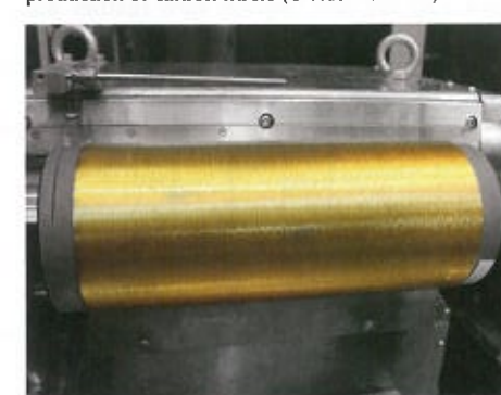
PAN fibers are the perfect precursor material for the production of carbon fibers (© Fraunhofer IAP)
