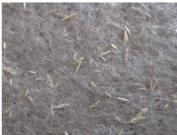
PLA non-woven felt with grass seed incorporated in 3D structure - demonstrator - DS Textiles
