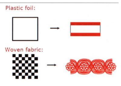
not evident for the active plasma species to penetrate into this structure, and thus, to ensure proper treatment throughout the textile. Several studies regarding this topic have been conducted. Crucial parameters are the gas pressure at which the plasma discharge is operated and, logically, the structure (thickness, density) of the textile material to be treated.
