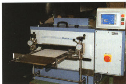
Fig. 1: the new Mathis coating and impregnation equipment
