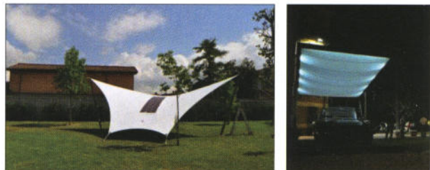
Figure 5: picture of two demonstrators showing the feasibility of combining textile membranes with energy harvesting via photovoltaic cells. Involved partners: Sioen, D'Appollonia, Canobbio.
