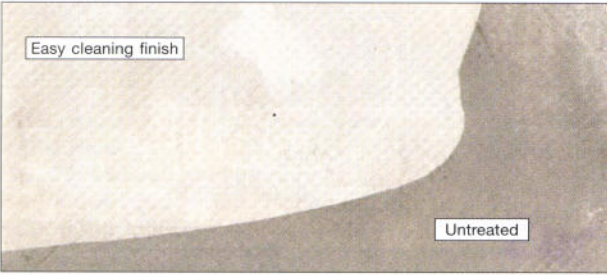
Figure 3: soiled and cleaned membrane which is partially treated with the new top coatings. The influence of the top coat can be clearly seen (partners: Sioen and Centexbel)
