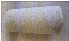
Figure 2: basalt / polymer roving
