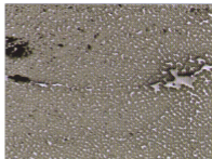
Figure 6: basalt / polyester composite structure
